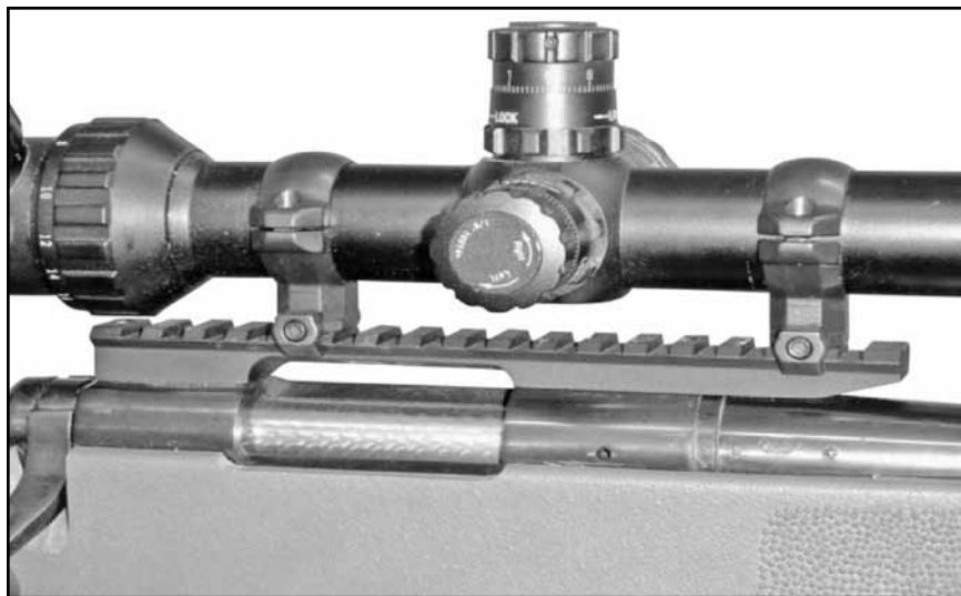
TRS-1 scope mounted on a tactical rifle using Millett Angle-Loc™ rings and Picatinny rail.
